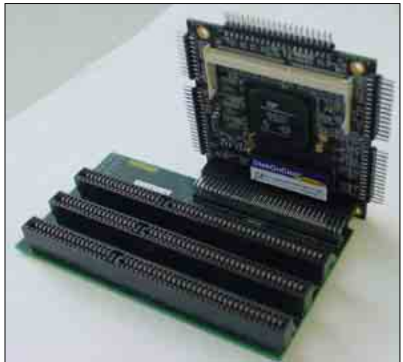
Figure 10. The MZ104 Plugged into a 16-Bit ISA Bus Passive Backplane
