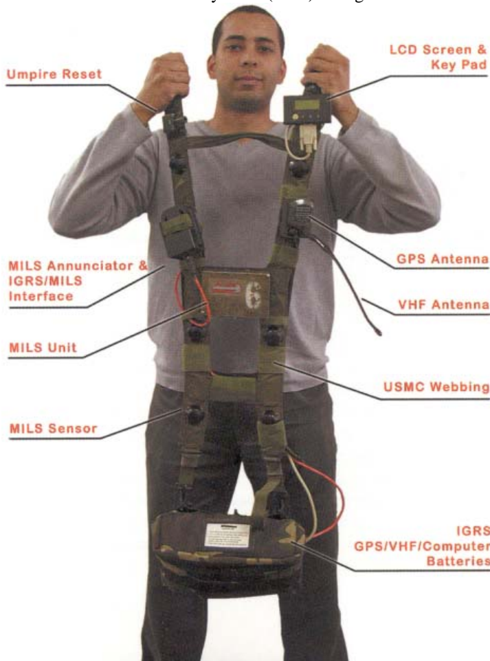
Figure 4 At slightly less than 11 lb, the IGRS/MILS unit is intentionally weighted to simulate a full ammunition load in addition to performing as a bi-directional digital gate to the Marine.
